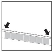
Set out a row of tiles across the wall and adjust so that equal cuts can be made in the corners. Mark the battern where the first tile is to go.
