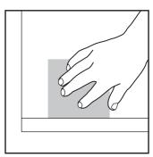
Start tiling at the mark on battern, placing tiles horizontally. Remove tile spacers before grouting.
