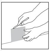
Find the lowest point on the floor line. Make a mark one tile height from the floor.
