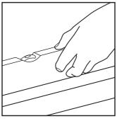
Nail a battern with a true edge on the mark. Check with spirit level to determine horizontal.
