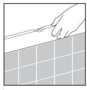
Check tiling regularly with a spirit level to keep work straight. Ensure that good contact with the adhesive is made.
