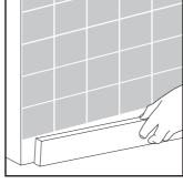
After adhesive has set, remove battern and fill in bottom row.
