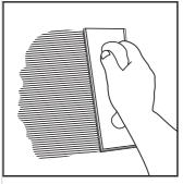
Use the straight edge of a notched trowel In a horizontal direction, notch the adheto spread adhesive on wall.
